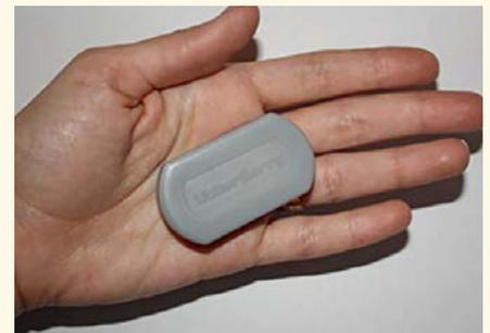
UtterBerry wireless sensors will revolutionize civil engineering instrumentation and monitoring, rendering the task easier to perform, with better measurement precision, and yielding dependable results in real time. They offer almost zero-power electronics, a powerful microprocessor, artificial intelligence and wireless communications. A sensor weighs 15 grammes and is about the size of a box of TicTacs.
